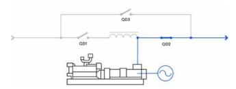
Independant Mode mtu Kinetic PowerPack provides energy as secondary power source, without interruption
